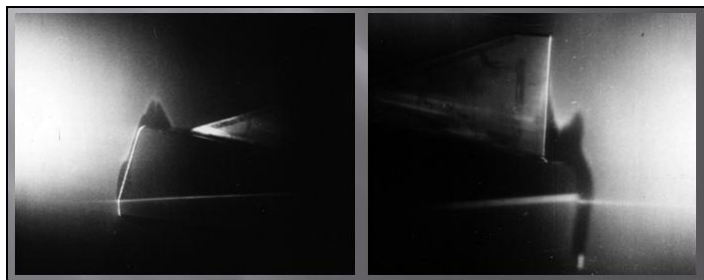
Figure 11. Vapor screen tests revealed unexpected but profound design features of the leading edge vortex flow fields.
