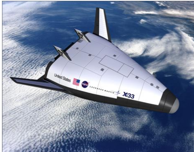
Figure 9. Initial fin arrangements were incompatible for aerodynamic stability.
