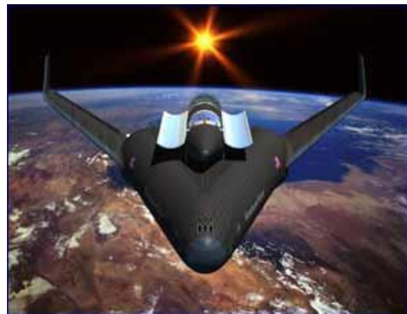
Figure 17. The full scale Venturestar/RLV appeared to be heading toward an external payload bay, possible to create more internal propellant volume.
