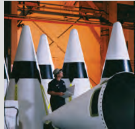
Orbital ATK's Aerospace Structures Division uses proven hand layup techniques to produce GEM 60 nose cones
