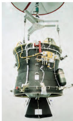
Lunar Prospector Size With Lifting Beam Tooling for Stage/Motor Handling
