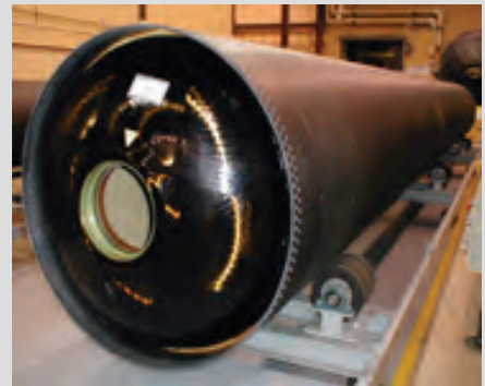
GEM cases are produced using advanced filament winding techniques developed and refined by Orbital ATK's Aerospace Structures Division for over 40 years
