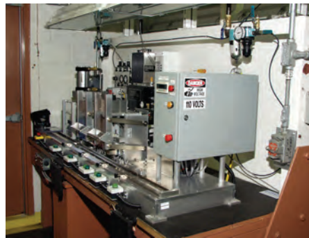
SCB Initiator Semi automated Manufacturing Line
