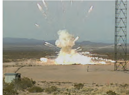
STAR 48 Destruct Test Using Model 2011 CSC
