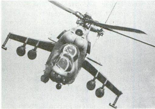
Mi-24/HIND E with Tube-Launched Anti-Tank Guided Missiles
